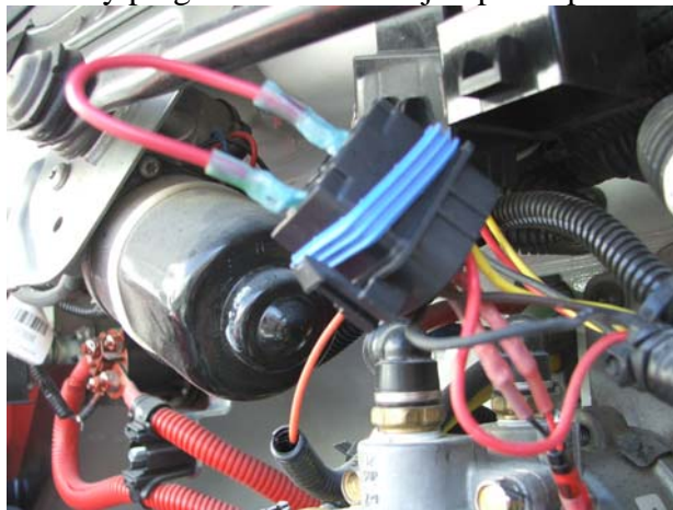
Relay plug shown with the jumper in place.
