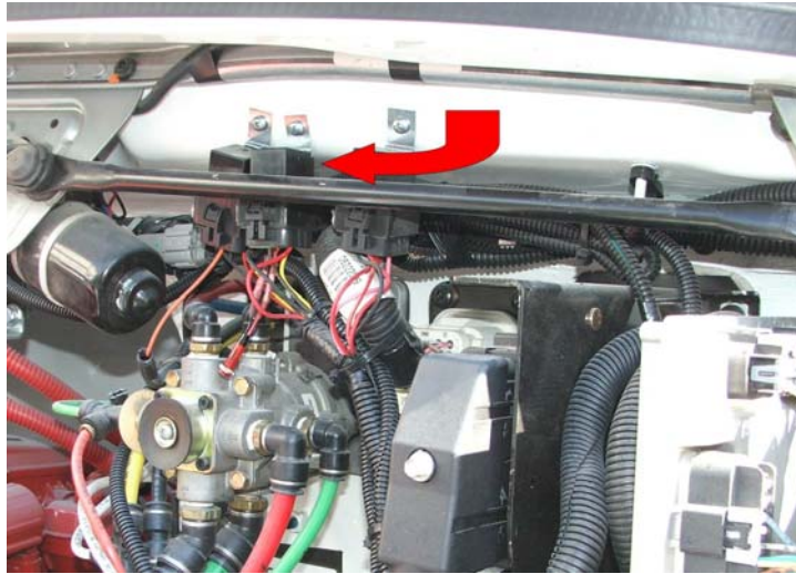
Relay plug shown with the jumper in place.
